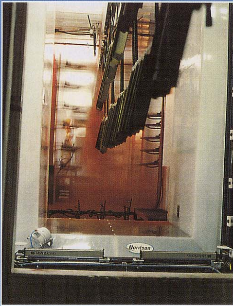
Electronic sensors identify the part before application begins inside the coating booth.
