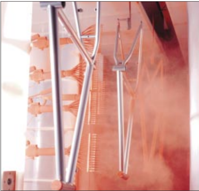
The powder colorcoat is applied with Tribomatic II powder guns (left). After the colorcoat is cured, a powder clearcoat is applied in a Horizon 400 booth (right).
