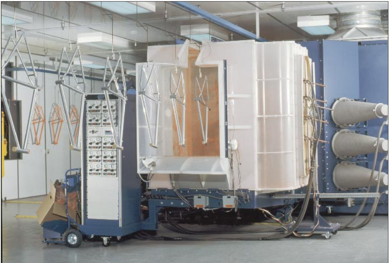
Bicycle frames are colorcoated in the CK booth (above). Three horizontal separators, attached to the right side of the booth, separate the reclaimed powder from the air. The separators allow easy access for cleaning.
