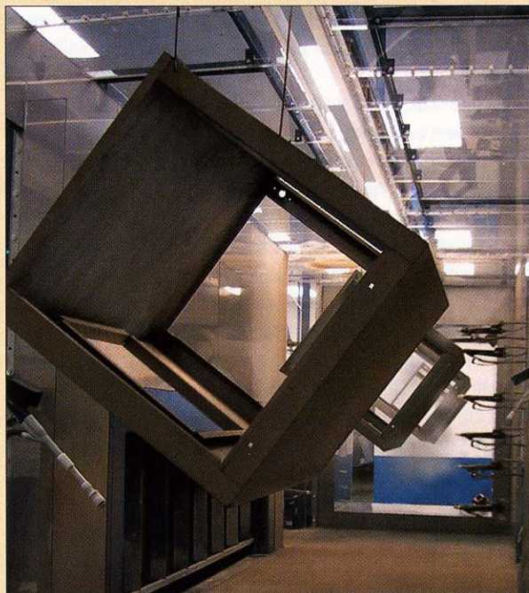
By replacing an old powder spray system, Essick Air Products achieved a cleaner spraying area and made other improvements in the coating process, while cutting powder use.
