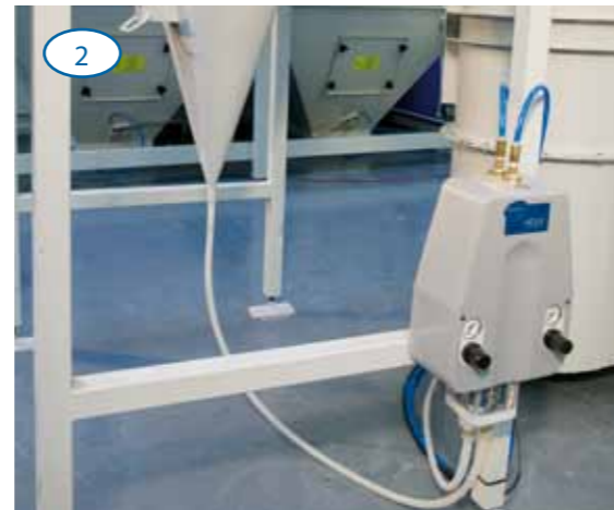
2 Prodigy® HDLV® dense phase circulation system continuously returns powder back to the feed centre.
