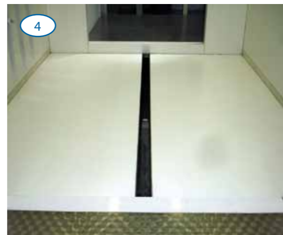
4 Booth base manufactured from Nordson Apogee® composite material with single extract duct along the length of the booth.
